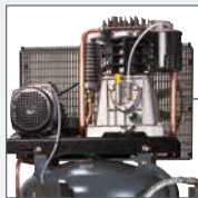
High-performance two-stage 2-cylinder power unit
